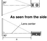
a is the distance (m) between the lens and the screen, and corresponds to a range of 1.07 m to 11.09 m.
